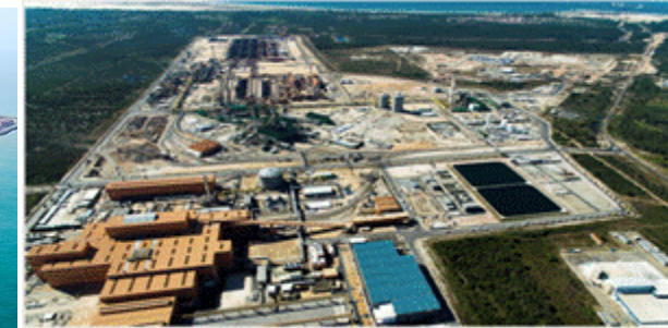
1 BF and 2 BOFs with 3Mt annual slab capacity
