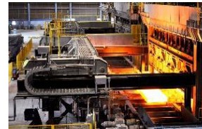
Hot Strip Mill (HSM) State-of-the-art HSM designed to roll AHSS, Line Pipe, & Stainless products
