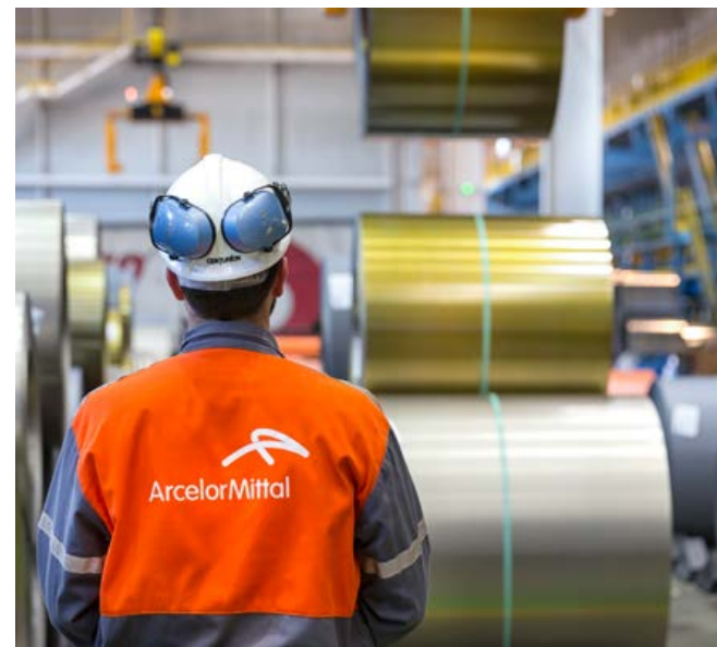
Varnished electrical steel coil being moved by crane ↑
