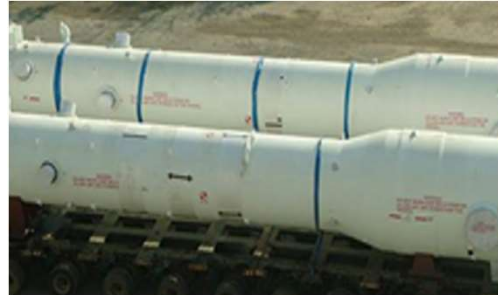
Nuclear Power Plant (Steam Generator) 16Mo3 - 1,200MT
